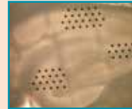
Hippocampal slice placed on the MED-P5001A
